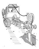
Depending on the size and number of conduit or fiber cables used for placing in a single pass, this method is very productive with less material handling. One or more reels are mounted on the plow and are guided safely over the plow tractor and fed directly into the plow chute. When the end of the reel or reels is reached, the tails are brought up and eventually coupled or joined to the starting ends of the next reel or reels.
